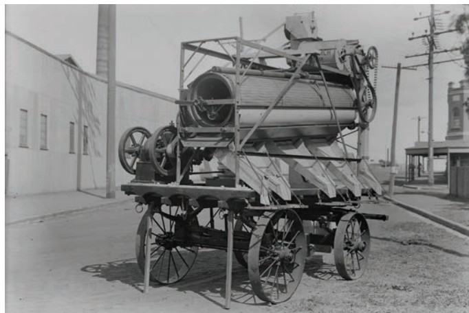
Photo of seed grading machine mounted on a wagon made by Clyde Engineering of Granville, NSW. Clyde Collection, MAAS Collection
