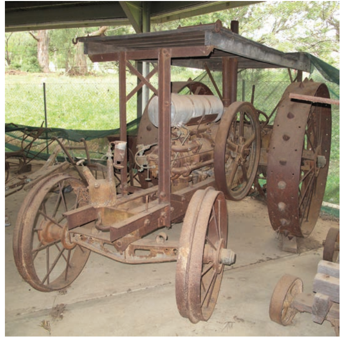
An early oil engine tractor known as a 'hit and miss'.
