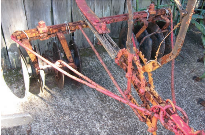
A good example of painted metal corroding from exposure to moisture and high humidity.
