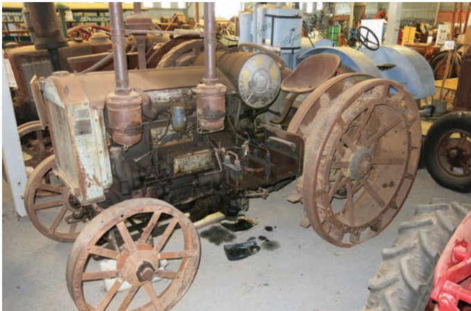
When storing an internal combustion engine, drain oil and replace it with inhibitors to prevent corrosion.
