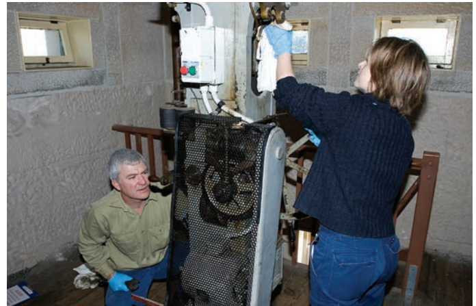
Removing an old wax coating and reapplying a fresh coat on Sydney Observatory's time ball mechanism. MAAS Collection
