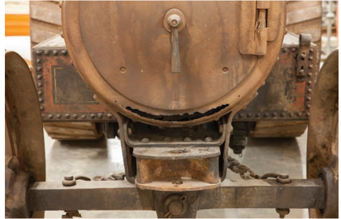
Moisture from the open chimney and ash in the smokebox has corroded this 1904 McLaren steam traction engine.
