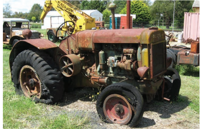
Rubber tyres perish over time, causing further deterioration to the machine. Axle stands will take the load off the machine.
