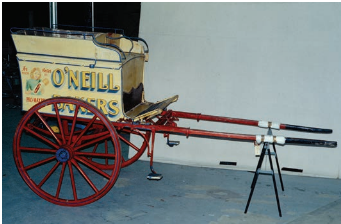
Stands help support the structure of this bread cart to prevent straining and damage. MAAS Collection
