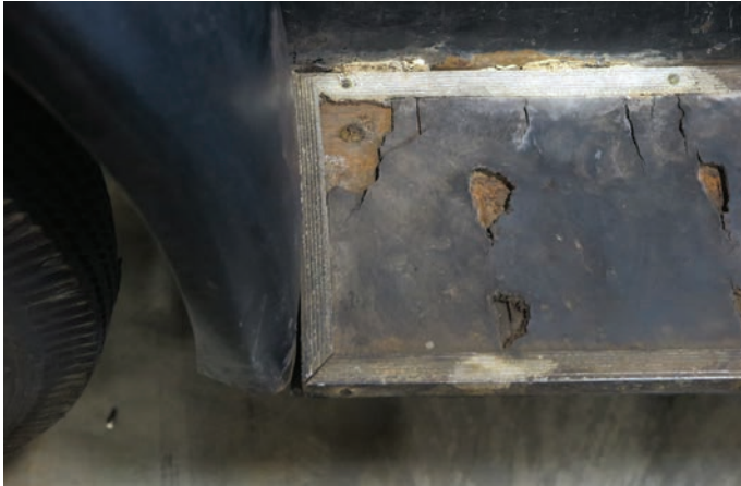
Exposure to the elements, particularly light, will damage surfaces such as the rubber of this car's running board.
