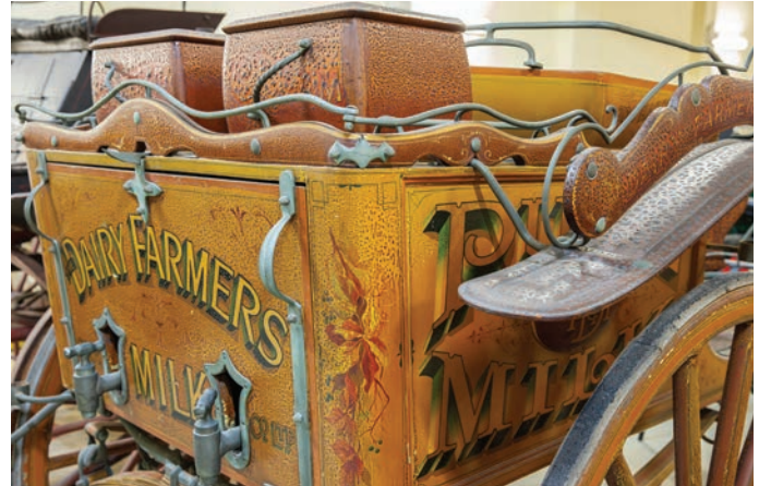
Exposure to light and heat has caused the shellac to blister on this 1930s milk cart. MAAS Collection
