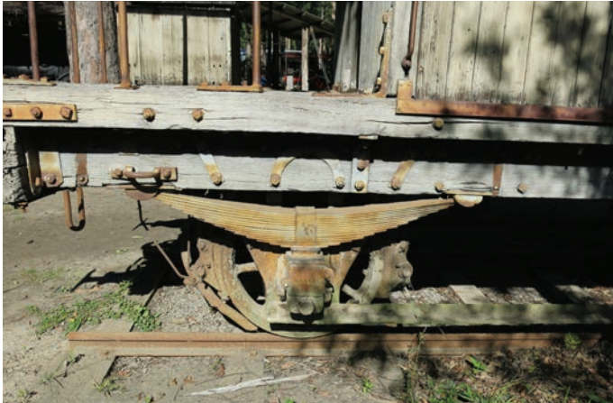
Evidence of wood splitting from continual expanding and contracting.
